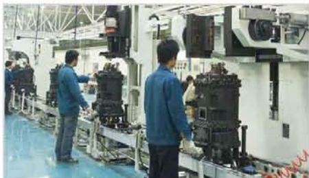
变速箱转配线 TRANSMISSION ASSEMBLY LINE
